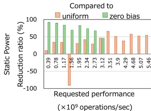
Fig. 11 Static power reduction ratio compared to the uniform and the zero bias cases ( $VDD = 0.55$  V)
